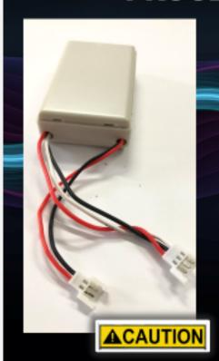
The Indicator light on the battery should be at the zipper end of the pouch. When on, a green light will glow indicating the battery is charged and blinks red when the battery needs to be re-charged. Be careful when changing the battery, each wire is different so therefore installation should be easy and error free. The wiring is short inside the glove so use caution when installing the battery and don't pull hard on the wires as this could damage the G.L.O.V.E.s connector and internal wiring.
