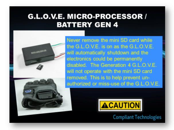
To download the mini SD card to the computer simply make sure the G.L.O.V.E. is off. Remove the SD card from the Battery/Micro-Processor and slide the mini SD card into the provided reader.
