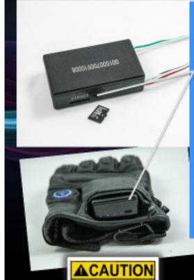
The battery indicator lights and charging port should be at the zipper end of the G.L.O.V.E. pouch and the serial number on the side oriented up. Be careful when removing and installing the B-MP. Do not grab the wires but each connector. When installing make sure all prongs go into each connector properly or the G.L.O.V.E. will not function. The wiring inside the G.L.O.V.E. is short so use caution when installing the B-MP and don't pull on the wires as this could damage internal connections.
